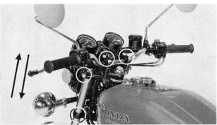
Fig. 2-11 (1) Checking front suspension
