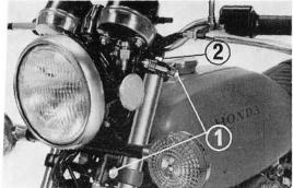
Fig 4-2 ① Front fork securing bolt
