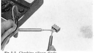
Fig. 5-5 Checking silicon diode
