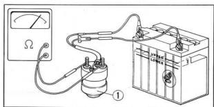
Fig. 5-30 (1) Starting magnetic switch
