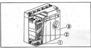
Fig. 5-32 ① Sediment ② Plates
