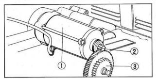
Fig. 5-22 ① Starting motor ② Starting motor shaft gear
