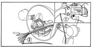
Fig. 5-41 ① Starter switch
