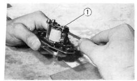
1 (1) Checking point gap with a feeler gauge
