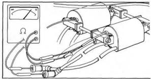
Fig. 5-3 Checking ignition coil for continuity
