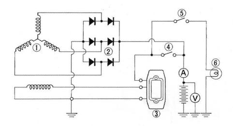
Fig. 5-12 Charging test circuit
