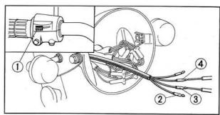
Fig. 5-38 ① Turn signal control switch
