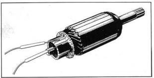
Fig. 5-27 Checking armature coil for continuity
