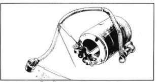
Fig. 5-26 Checking field coil for continuity
