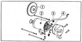
Fig. 5-24 ① Starting motor reduction gear
