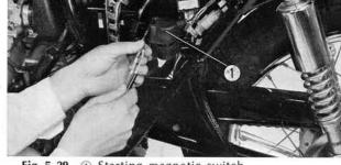
Fig. 5-29 ① Starting magnetic switch
