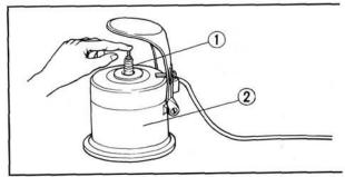
Fig. 5-6 ① Spark plug ② Plug cleaner
