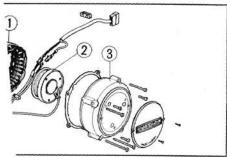
fig. 5-13 1 Stator coil 2 Field coil 3 Dynamo cover
