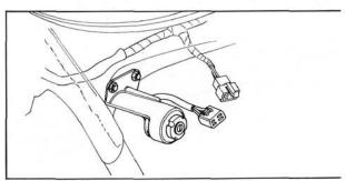
Fig. 5-34 Checking main switch
