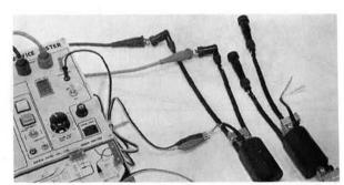
Fig. 5-4 Ignition coil performance test
