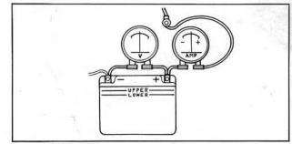
Fig. 5-11 Charging test
