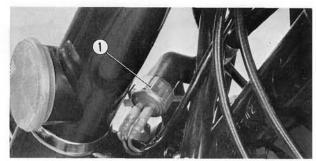
Fig. 5-35 ① Front stop switch
