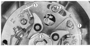
Fig. 5-7 ① Breaker point gap ② Matching mark
