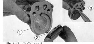
Fig. 4-16 ① Caliper B ② Pad B ③ Cotter pin
