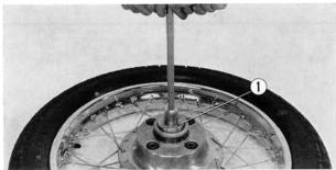
Fig. 4-29 (1) Bearing retainer wrench
