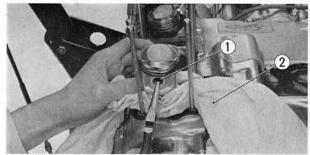
Fig. 3-11 ① Piston pin clip ② Waste cloth
