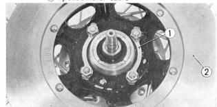
Fig. 4-3 (1) Lock washer (2) Brake disc
