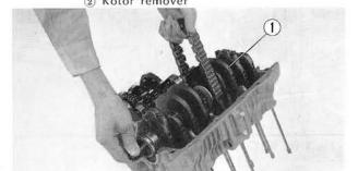
Fig. 3-65 ① Crankshaft
