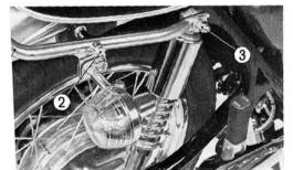
fig. 4-55 ① Rear bumper ② 8 mm bolt
