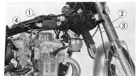
fig.4-40 ① Clutch cable ③ Speedometer cable ② Tachometer cable ④ Throttle cables
