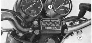
Fig. 4-36 (1) Upper handle holder (2) Steering handlebar
