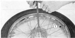
Fig. 4-4 (1) Bearing retainer wrench
