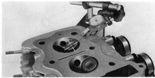
Fig. 3-14 Checking valve-to-valve guide clearance
