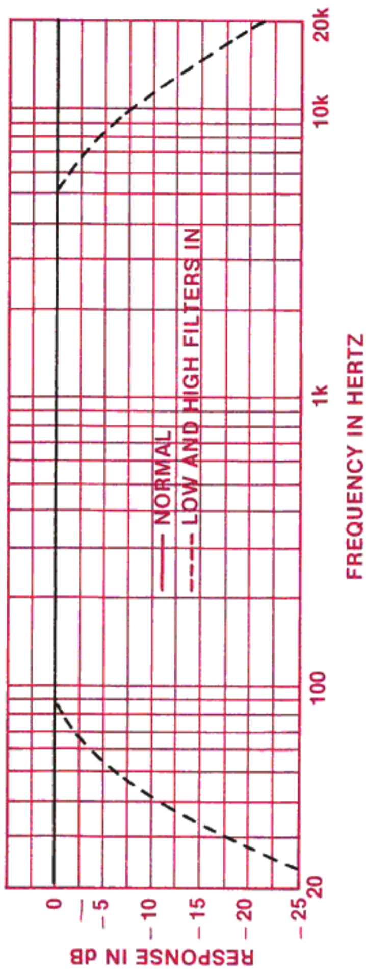
LOW AND HIGH FREQUENCY FILTER CHARACTERISTICS
