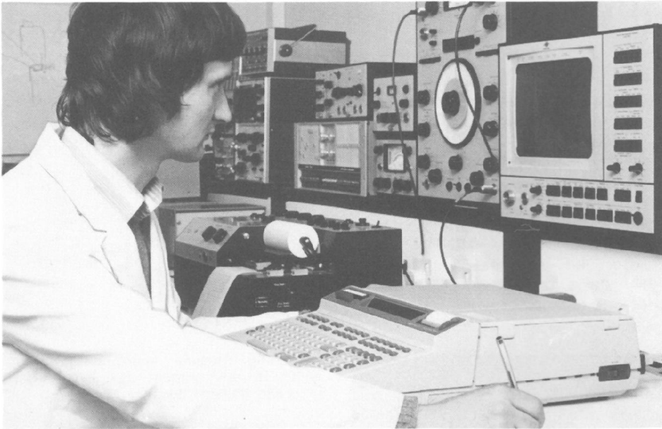
Measuring energy versus time response of the 801 using a B&K 2031 spectrum analyser interfaced to HP 9825A desk-top computer.
