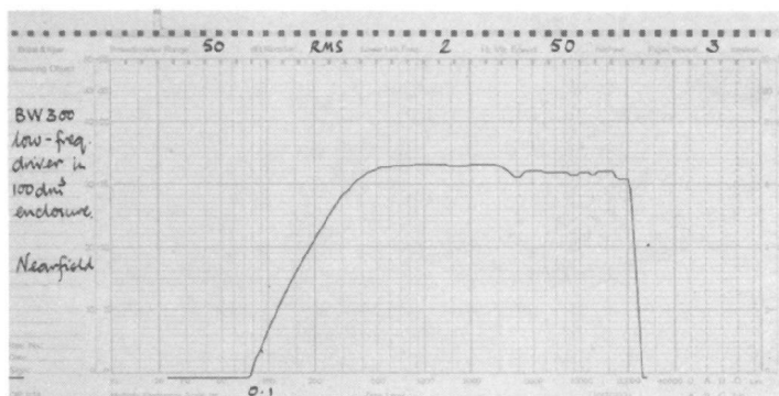
Fig. 10 Amplitude/frequency response of low-frequency system measured using the nearfield microphone technique.
